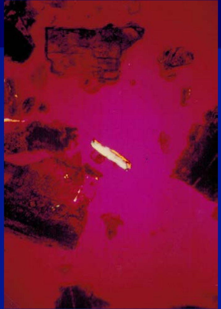
Gypsum falls out from broken salt crystals
