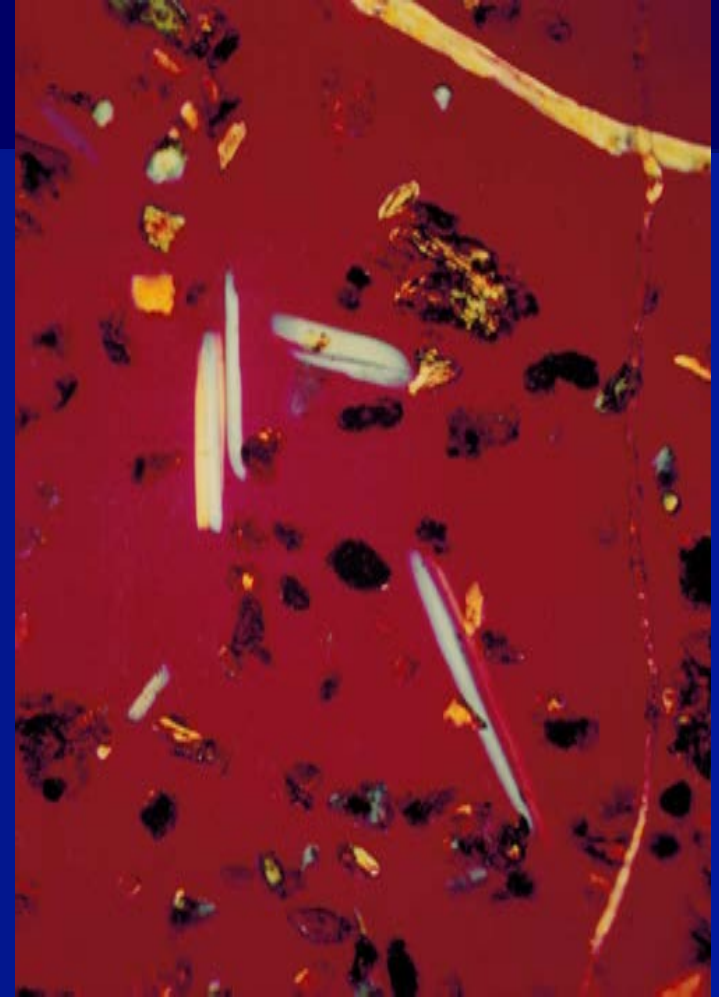
Excessive washing dissolves salt leaving only gypsum and insolubles
